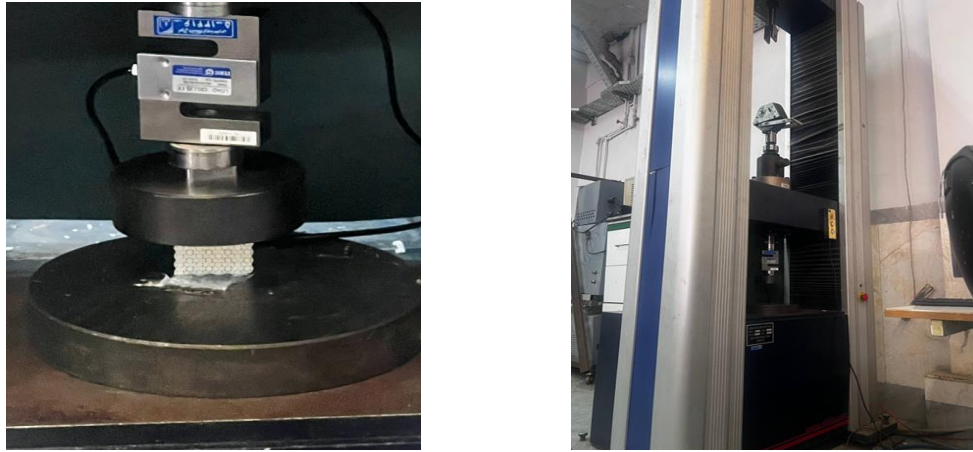
Figure 3. Compression test machine and the honeycomb specimen under compressive loading
