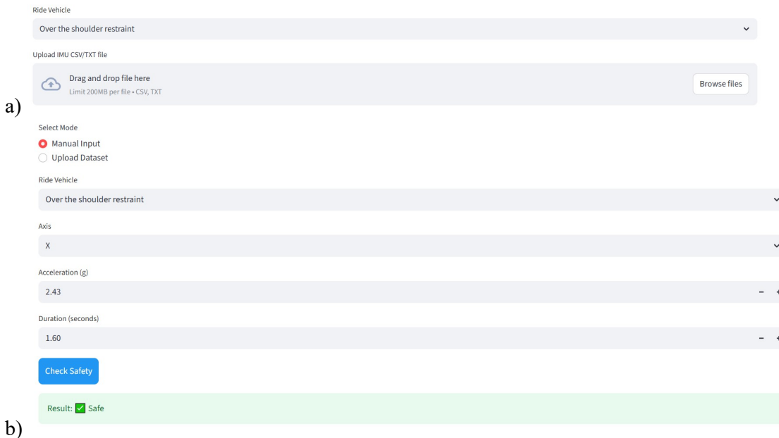
Figure 2. User Interface of the developed standard-compliant framework for acceleration safety check when using amusement rides: a) signal processing mode b) manual mode
