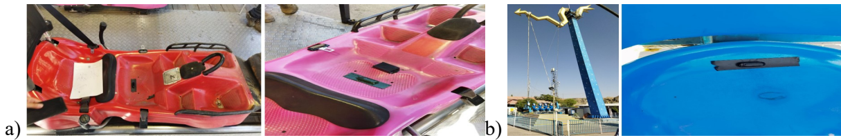
Figure 4. IMU Sensor attached to the rides in data collection process: a) Alpine Coaster b) Lightning ride
