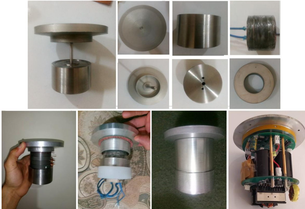
Figure 16: Components of the pinger along with the electronic circuit.
