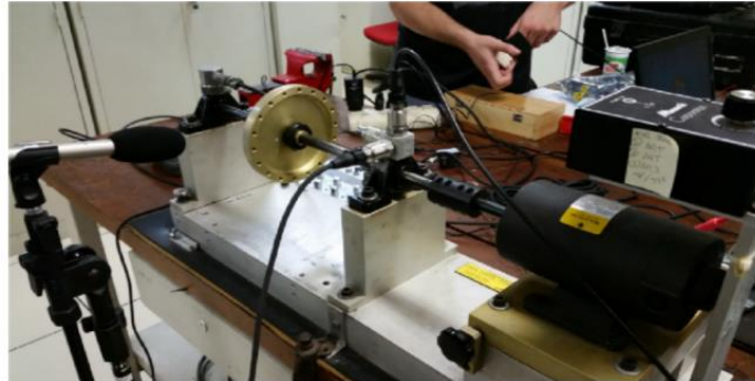
Fig. 1: The rotor-bearing test rig used to collect the MAFAULDA dataset.
