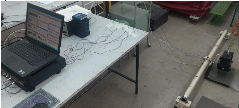
Figure 2. Experimental setup for bolt loosening test
