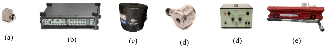
Figure 3. Equipment for conducting the experiment: a) Accelerometer b) Pulse Data Acquisition c) Shaker d) Force transducer e) Amplifier f) Torque Wrench
