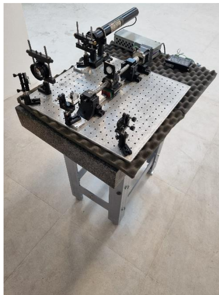
Figure 5. Optical setup mounted on a granite surface with dampers.
