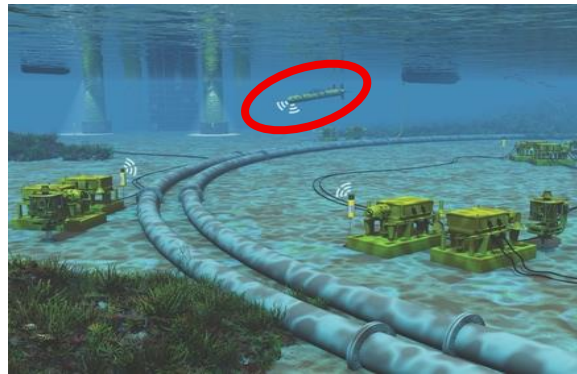
Figure 2. Schematic of a deep-sea AUV performing subsea oil and gas operations, illustrating typical underwater acoustic communication links between the AUV, surface vessels, and subsea infrastructure.[7]
